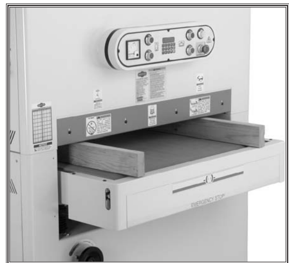
Figure 52. Gauge boards placed under pressure rollers.
